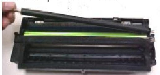
Fig. (E-210) 10 – Retirando o PCR
